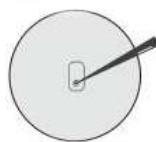
Use a tool (such as a Sim card pin, mini screwdriver, fine pin) to press the elastic button while pushing the back cover down.
