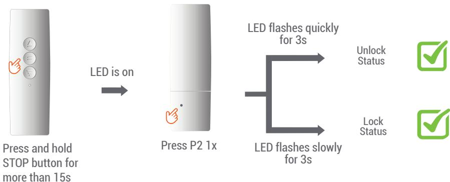
**⚠NOTE** With the lock function you can not program functions in which you need two buttons like limit settings and change direction.
